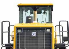
The panorama rear windscreen with rear wiper and the reversing sensor equipped ensure good visual field and safe reversing.
